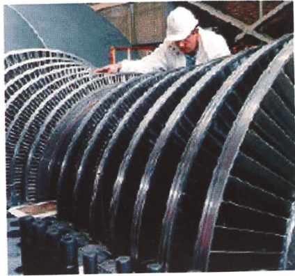
Fig.10 Turbine with integrally shrouded blades.
