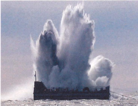
Figure 3. Shock Test Barge.
