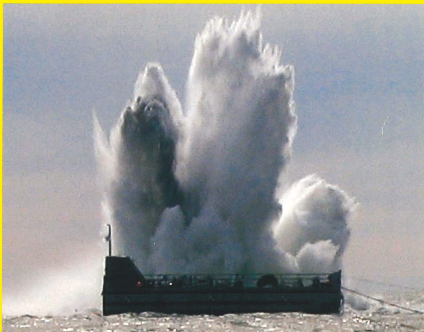
Shock Test Barge, developed by the Finnish Navy and VTT for heavy duty underwater shock field tests
