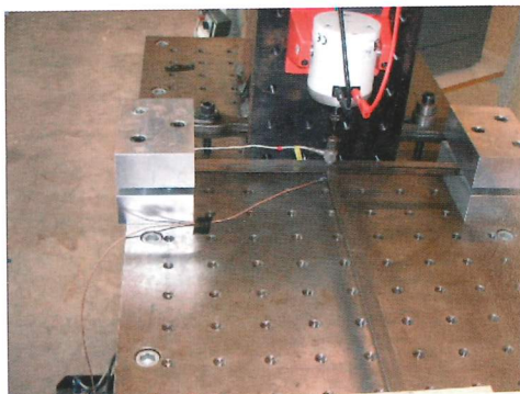
Figure 5.3: The complete setup for the experimental test. The structure is fixed to a rigid table and a shaker is used to excite the structure.
