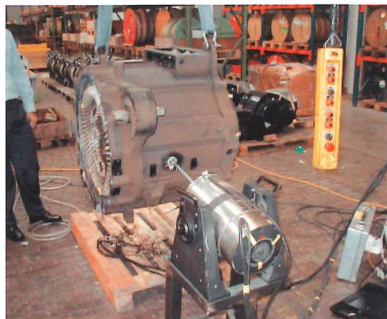
Multi-channel vibration measurements for determination of structural-dynamic properties
