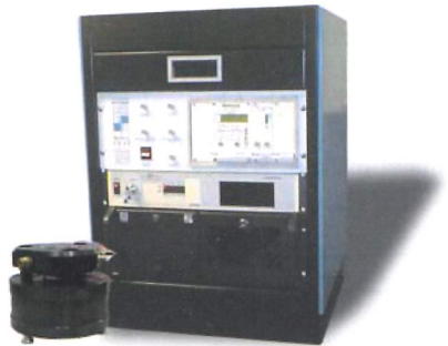
Figure 1: Accelerometer Calibration Workstation next to an electrodynamic air bearing calibration shaker [1].
