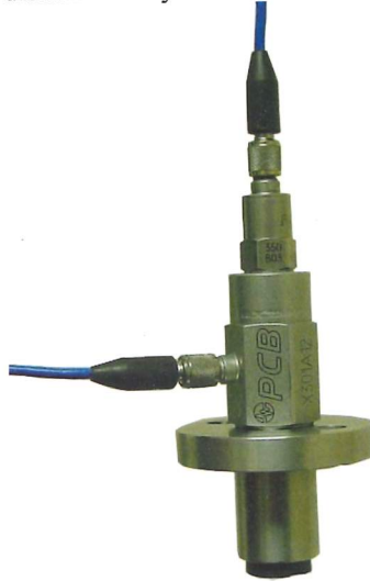
Figure 4: test transducer, reference transducer, and anvil mounting arrangement detail. Printed calibration certificates fulfilling the requirements set forth by ISO 17025 can be easily generated, and calibration results can be stored in open database format for ease of retrieval and data management. The system can also test accelerometers for other characteristics, such as zero shift, ringing, and nonlinearity. Figure 5 shows a typical screen shot of the measured shock and the calibration results produced with the pneumatic exciter described above.
